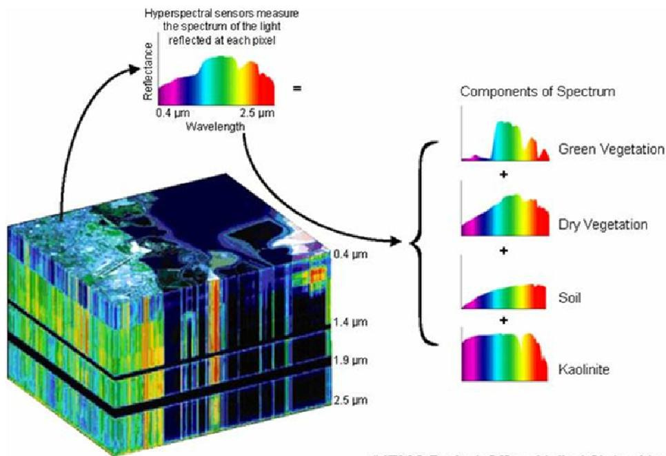
**Figure C8-1:** Hyperspectral data “cube” with examples of some spectral profiles
